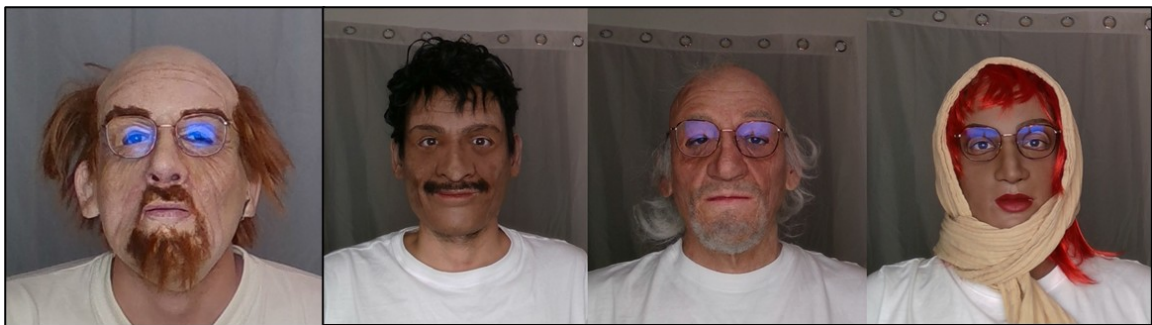
Figure E.18 – Examples of one high-quality latex mask attack (left) and three silicone mask attacks (right)
