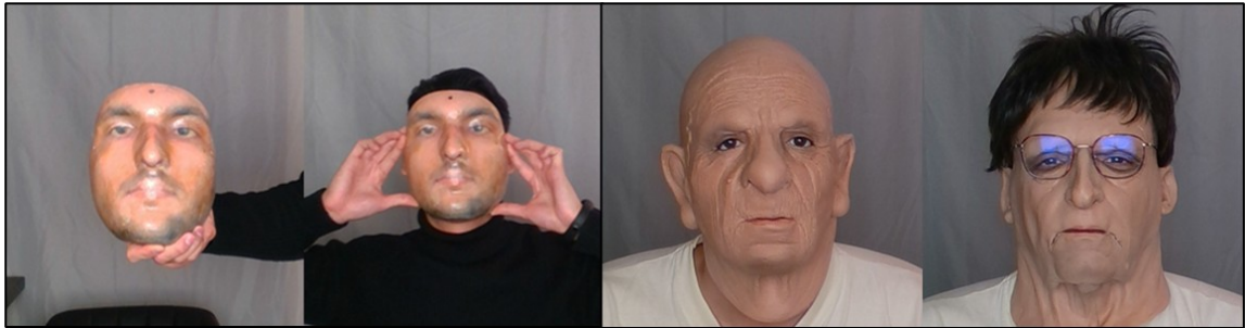
Figure E.17 – Examples of two 3D rigid mask attacks (left) and two latex mask attacks (right)
