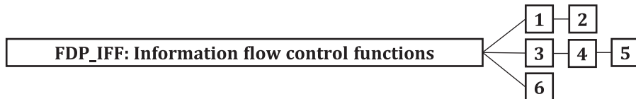
Figure 28 — FDP_IFF: Component leveling
